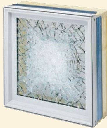
Figure 3. Impact-resistant window after sustaining the force of a nine-pound 2x4 shot at 34 miles per hour in testing. Courtesy of Pella Corporation.
